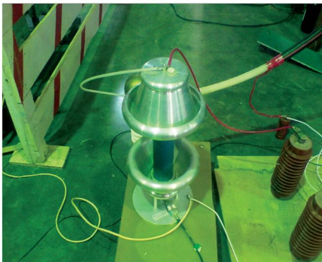
Figure A.1.2.4.5 Experimental set up for wire burn test for RHVPS
