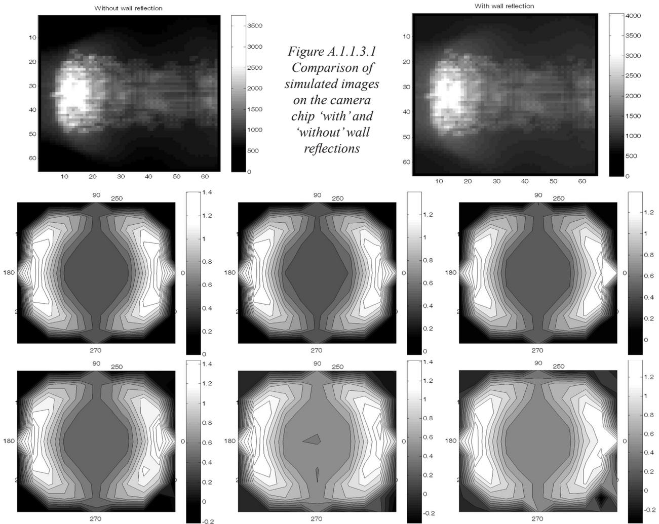
Figure A.1.1.3.1 Comparison of simulated images on the camera chip ‘with’ and ‘without’ wall reflections
