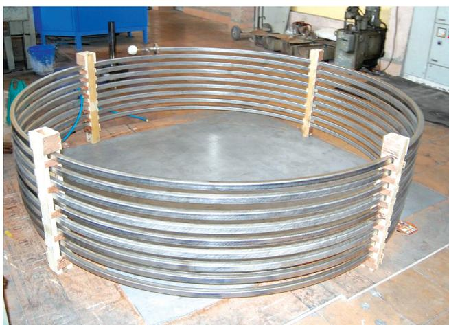
Figure A.2.2.1 30 kA CICC indigenously developed by IPR-AFD(BARC)
