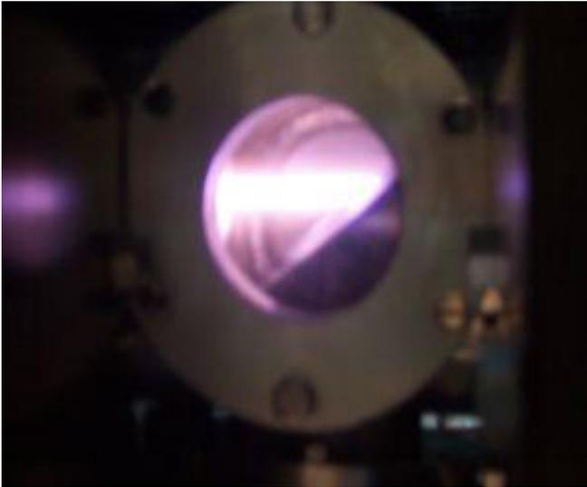
Figure A.3.4.2 Plasma (ion) beam falling on 45° reflector plate
