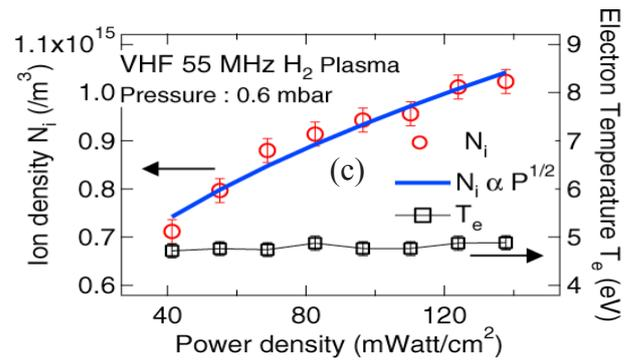
Figure A.5.2.1 Radial (a) ion density ( $N_i$ ) and (b) electron temperature ( $T_e$ ) profiles for VHF (55 MHz) and RF (13.56 MHz)  $\text{H}_2$  plasma at pressure 0.6 mbar with 40  $\text{mW/cm}^2$  in the same reactor. (c)  $N_i$  and  $T_e$  as a function of power density.
