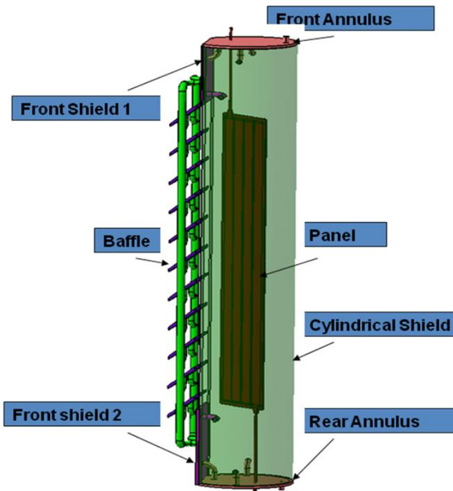
Figure A.2.3.2 CAD model of Cryopump
