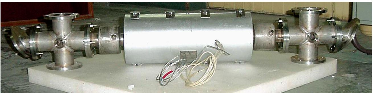
Figure A.3.5.1 Plasma chamber for PWFA being tested
