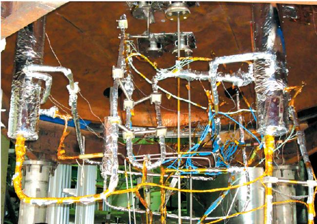
Figure A.1.2.2.4 Joint validation test Assembly in Test cryostat
