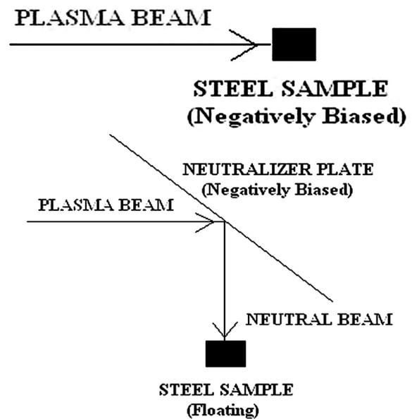
Figure A.3.4.1 (a) A steel sample being processed by plasma (ion) beam ; (b) being processed by neutral beam
