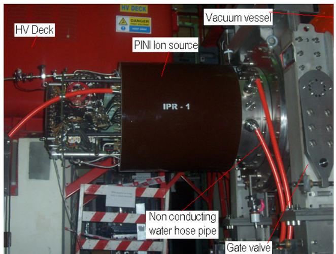
Figure A.1.2.4.4 PINI ion source is mounted on vacuum vessel
