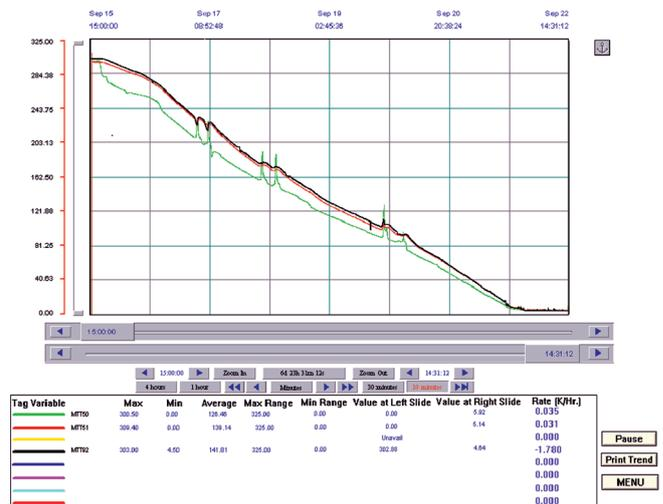
Figure A.1.2.2.3 Controlled cool-down of the Spare TF coil during the tests
