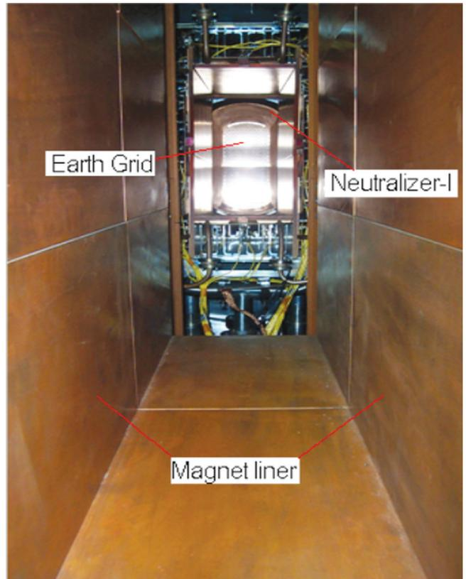
Figure A.1.2.4.3 View of magnet liner, neutralizer and earth grid under progress.
