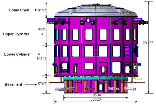
Figure B.2.5. Typical cryostat structure eliminate ribs inside the small cylinder) and supports layout, considering the upper bio-shield supported from the building. (2) Perform detailed structure analysis for penetrations under the operation and accident conditions.
