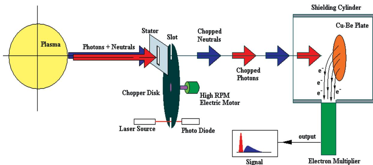
Figure A.1.1.3.6 Schematic of the Time-of-flight neutral particle analyzer planned for aditya tokamak
