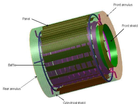
Figure A.2.3.1. Multipanel Cryosorption cryopump
