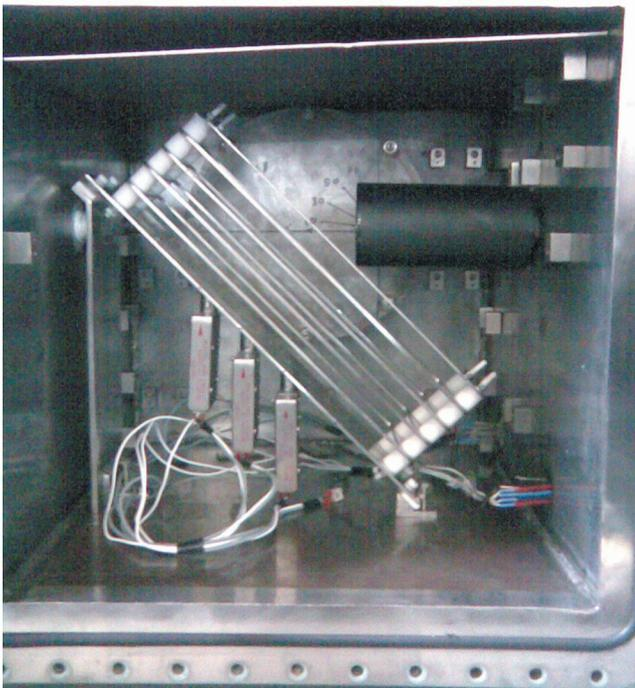
Figure A.1.1.3.4 Photograph of 45° Parallel Plate Electrostatic Energy Analyzer
