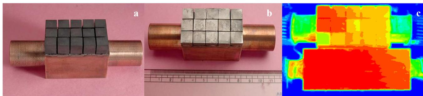
Figure A.2.1.1 Test mockup with (a) Graphite tiles brazed to CuCrZr copper alloy heat sink; (b) with Tungsten tiles brazed to CuCrZr copper alloy heat sink; (c) Comparison of temperature distribution on NAL test mock-up (top) with reference test mock-up (bottom) during transient IR-Thermography at  $t=20\text{sec}$  after switching from cold water ( $28^\circ\text{C}$ ) to hot water ( $85^\circ\text{C}$ ).
