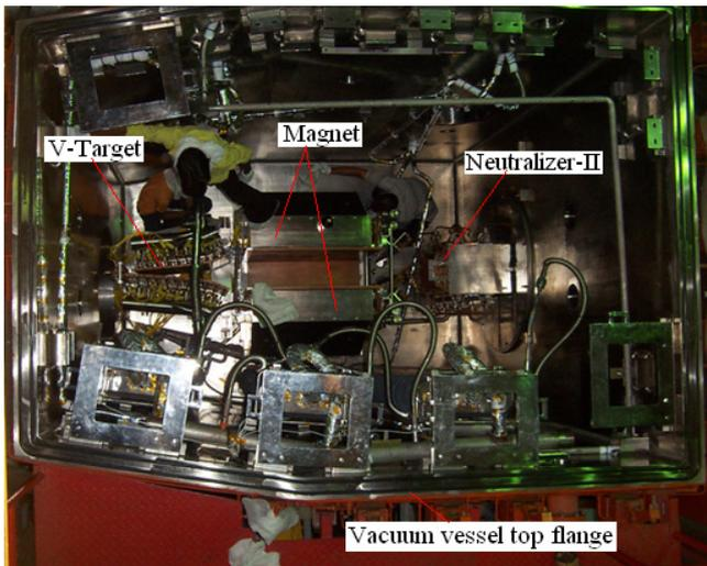
Figure A.1.2.4.2 View of the NBI components placed inside the vacuum vessel.
