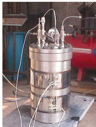
Figure B.2.4. Autoclave design for immersion tests
