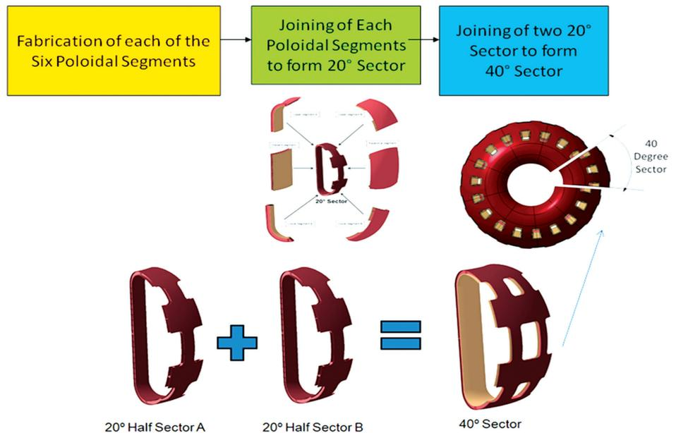
Figure A.2.3.3 Plan for fabrication of 40° sector
