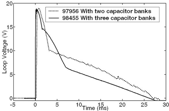
Figure A.1.1.2.2(a) Comparison of Loop voltage using old and upgraded capacitor bank
