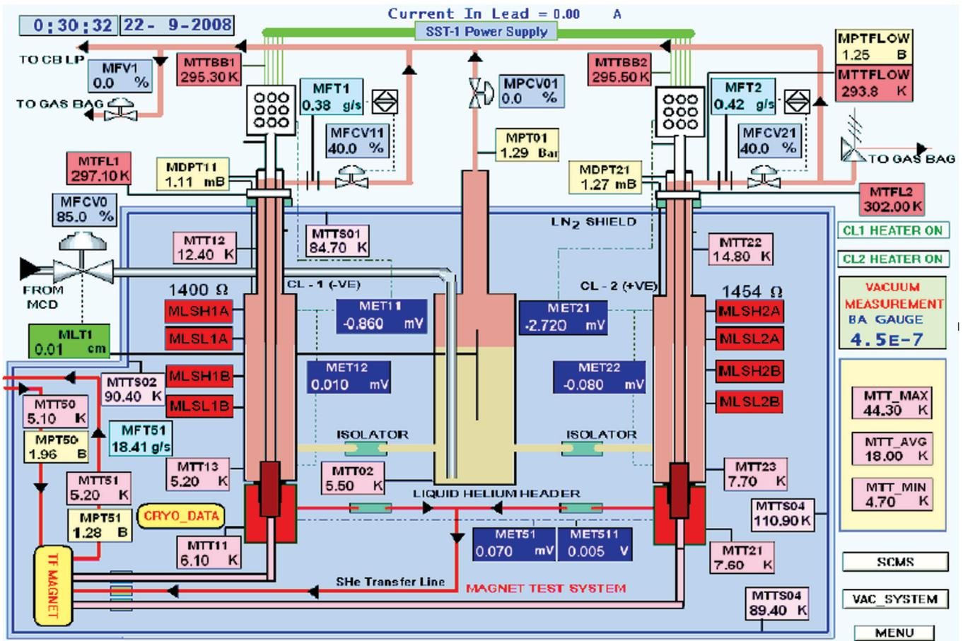
Figure A.1.2.2.2 MIMIC developed and used for the Current Feeder System during the test
