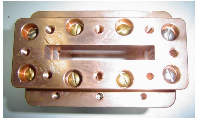
Figure A.1.2.4.1(a) photograph of proto-type three-step waveguide transformer
