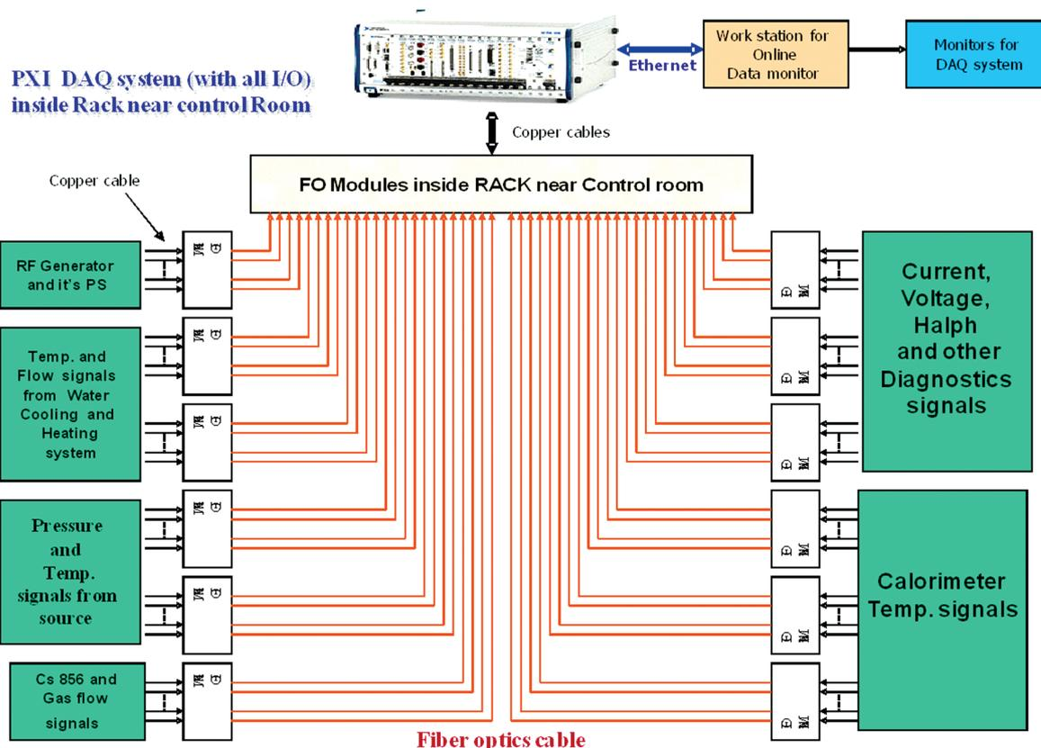
Figure A.2.5.2 PXI based Data Acquisition system with fiber optic link in each channel
