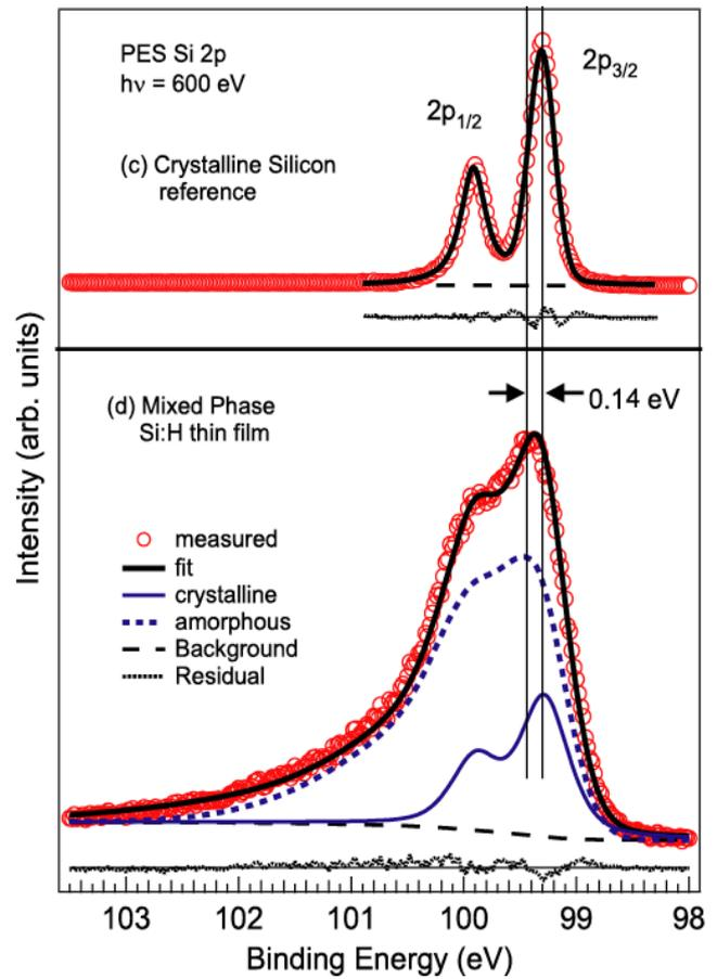
Figure A.5.2.2 (a) AFM image shows  $\mu\text{-Si:H}$  crystallites embedded in  $a\text{-Si:H}$  matrix and (b) shows a line profile across two crystallites. Si 2p core level PES for (c) crystalline silicon reference sample and (d) mixed phase Si:H thin film.
