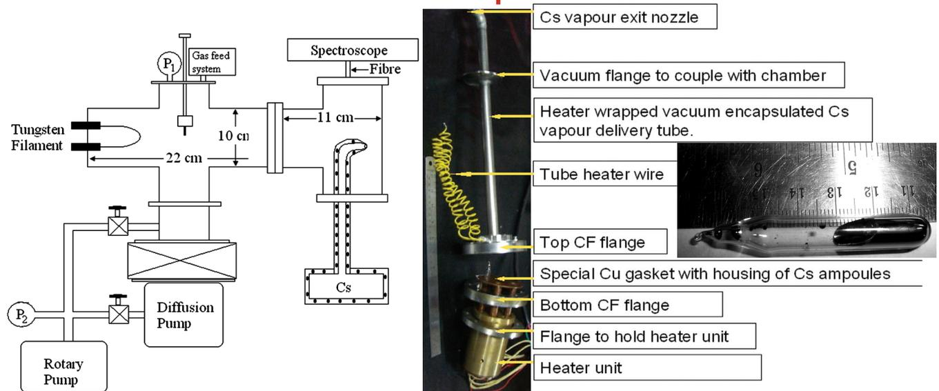
Figure A.2.5.1 Experimental setup of Cs oven experiments at IPR
