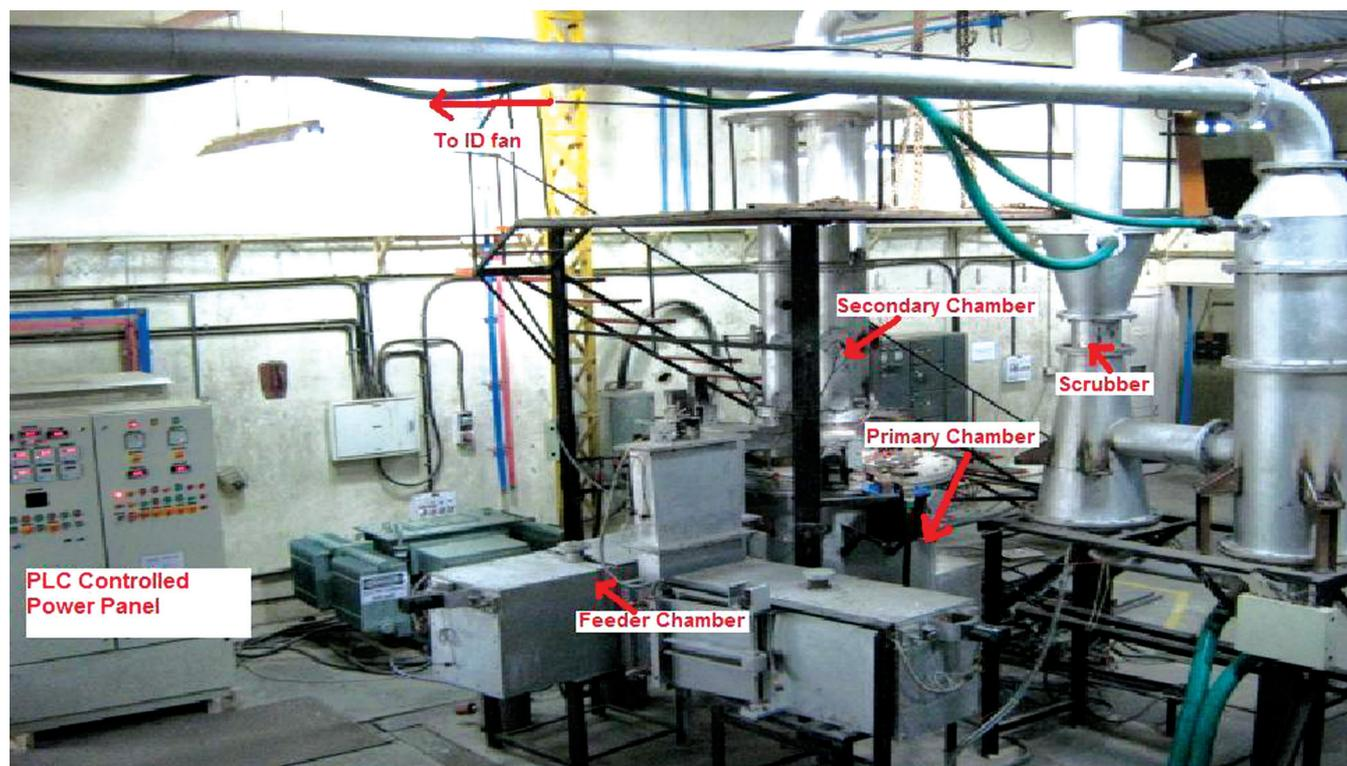
Figure A.5.1.1 Higher capacity plasma pyrolysis system as demonstrated and tested at FCIPT.
