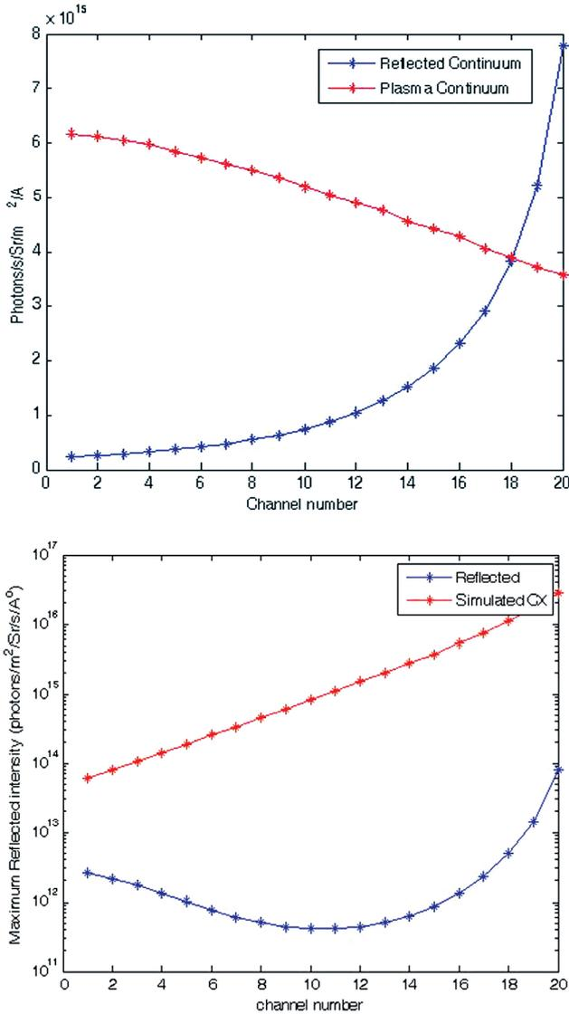
Figure A.1.1.3.3 Simulated and reflected continuum signals for ITER are shown in the top panel while both the CX signals are shown in the bottom panel.
