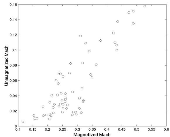
Figure A.1.1.5.2 Mach numbers measured simultaneously by the magnetized and unmagnetized Mach probes.
