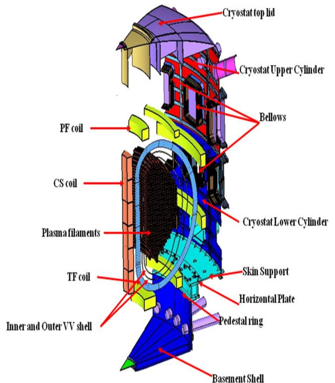
Figure B.2.6. 40 degree sector for Electro-Magnetic and structural analysis
