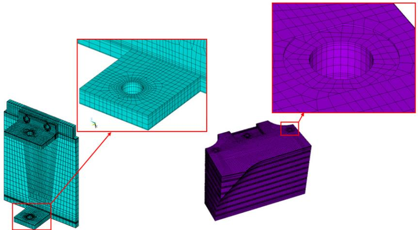
Figure B.2.2. Finte Element model of IWS block Row\_22\_A
