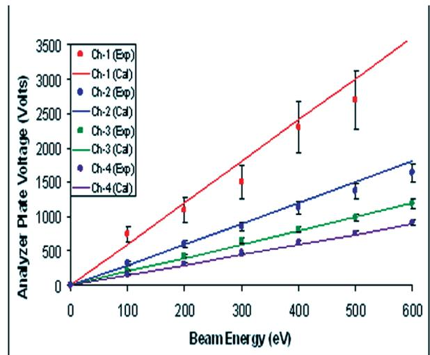
Figure A.1.1.3.5 4-Channel Calibration plot for 45° Parallel Plate Electrostatic Energy Analyzer
