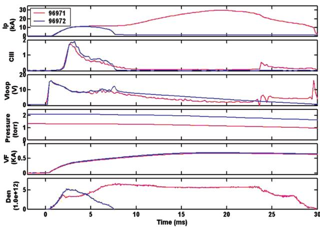
Figure A.1.1.2.3 (a) Failure of discharges at higher pressure. Insufficient burn through of CIII impurity at higher operating pressure. Red: low and Blue: high pressure
