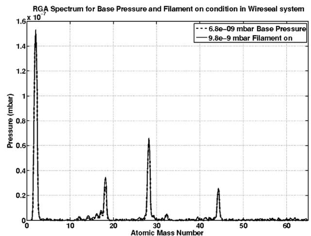
Figure A.3.3.1 RGA scan for Aluminum Wireseal (Solid line: Filament on, Dashed line: Base pressure)
