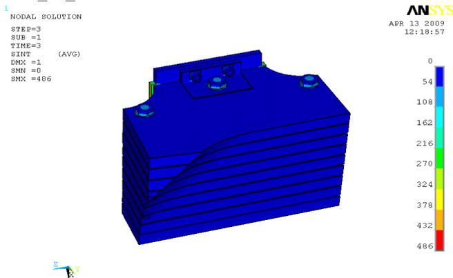
Figure B.2.3 Stress distribution on IWS block Row\_22\_A
