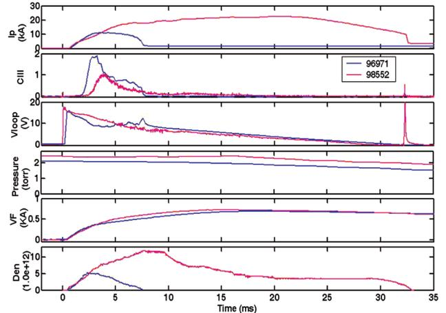
Figure A.1.1.2.3(b) Discharges at higher pressure with additional bank.: Red: high pressure ( $1.2 \times 10^{-4}$  torr) with additional bank, Blue: without additional bank
