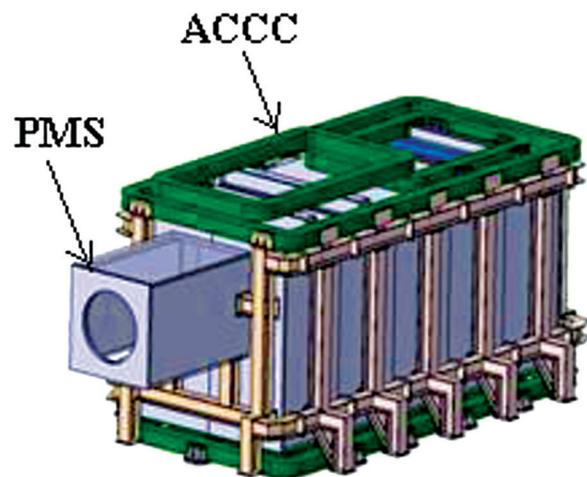
Figure B.2.12 Magnetic field reduction system
