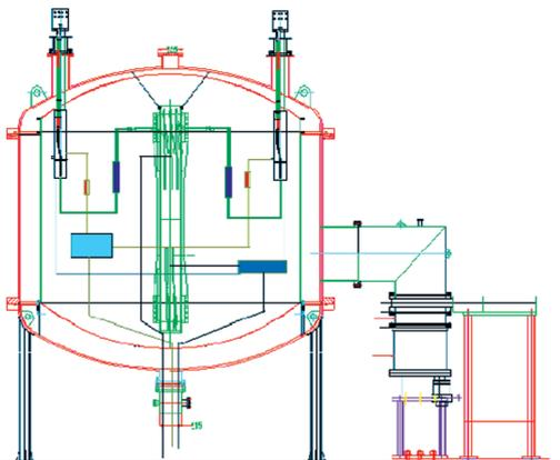
Figure A.1.2.2.1 Coil test assembly showing the current leads and vacuum system and some basic components
