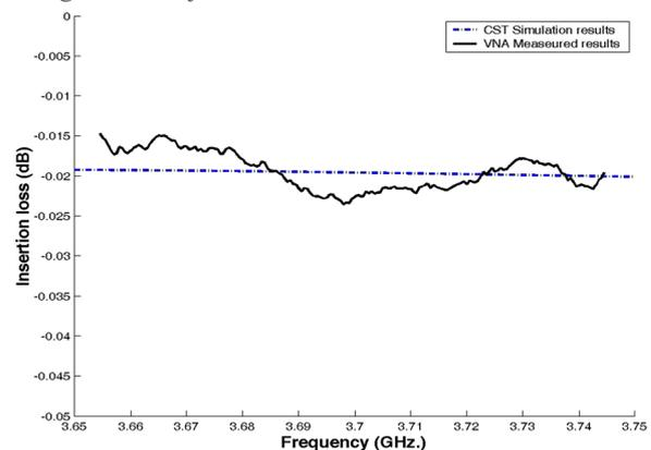
Figure A.1.2.4.1(b) The insertion loss measured using VNA is compared with CST simulation results for the proto-type waveguide transformer.
