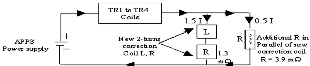
Figure A.1.1.2.1 Equivalent circuit for the correction coil
