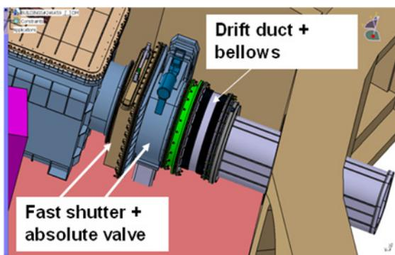
Figure B.2.11 Front-end Components
